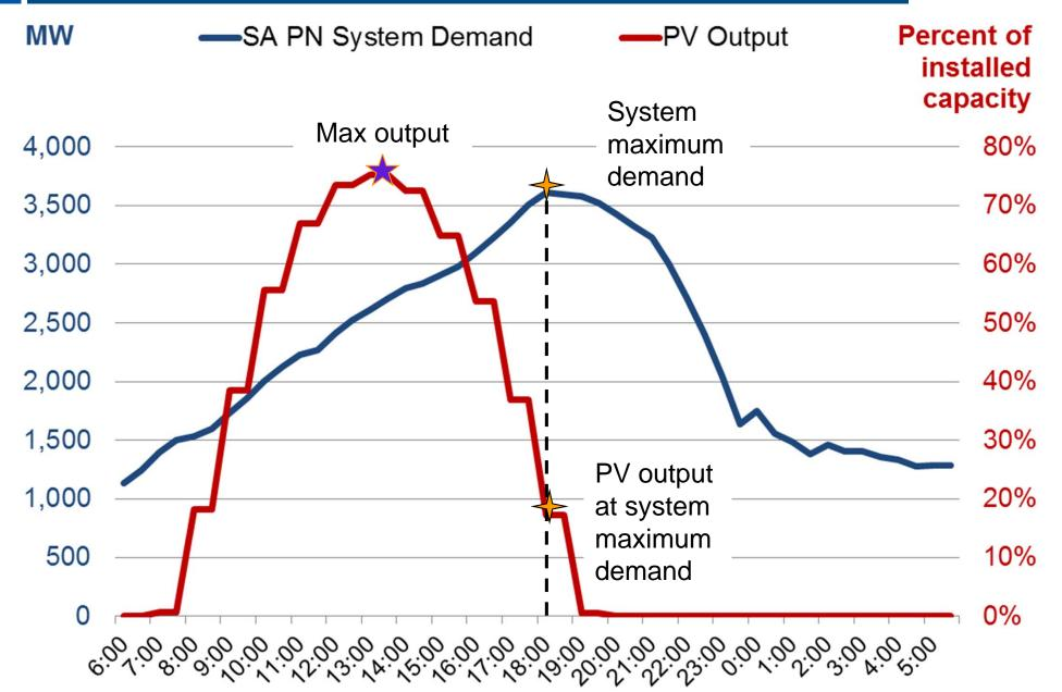
Note: The system maximum demand represented here is for SA Power Networks for 2011. The solar PV output is derived by NERA using the System Advisory Model and information on installed capacity published by the Clean Energy Regulator
