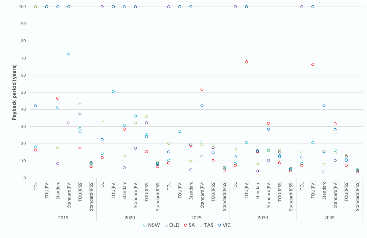
Figure 25: Discounted payback periods for mid-range battery costs, large-size commercial customer by end-use case, NEM states
