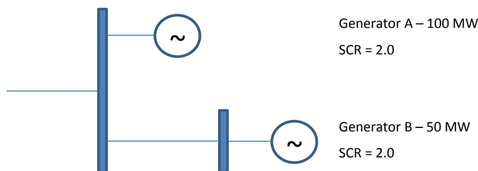
Required fault level to support operation of only Generator A = 200 MVA, ESCR = 2.0
