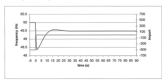
The power system frequency and the SA import during and immediately following the separation event are shown in the above graph.
