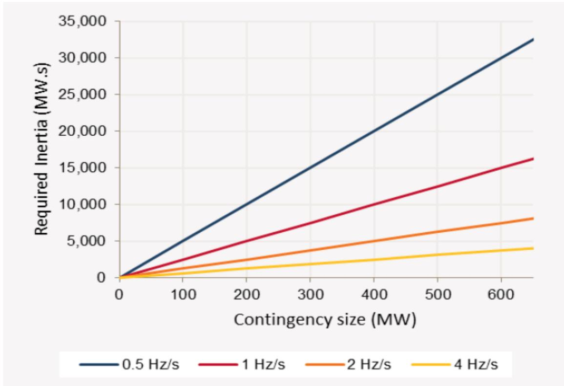
$$\text{RoCoF} = \frac{50\text{Hz} \times \text{Contingency size (MW)}}{2 \times \text{System inertia (MW.s)}}$$
