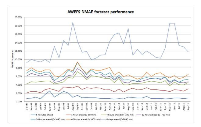
Figure 5.4 Accuracy of AWEFS (normalised mean absolute error)
