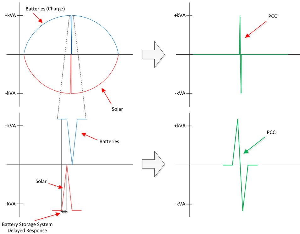
**Figure 1: Worst Case - Battery Control Delay Causing Import & Export Equal to the Solar Output**
