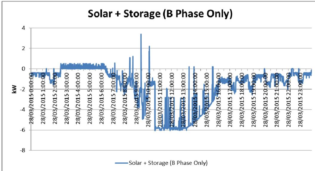
**Figure 3: Example of Battery Storage and PV Controlled for Load Leveling**
