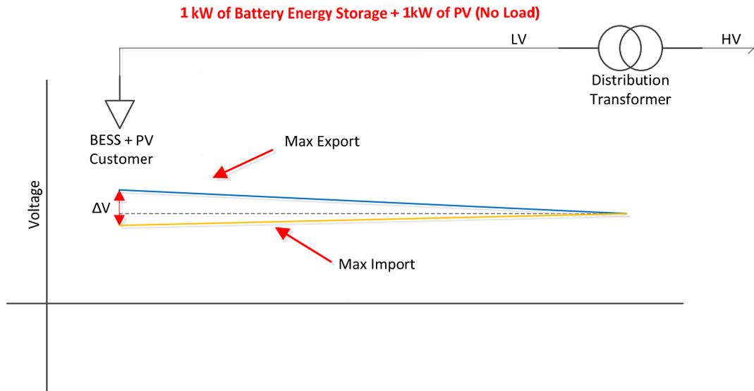
**Figure 6: Premise with 1kW of Battery Energy Storage and 1kW of PV (No Load) - Change in Voltage Profile**
