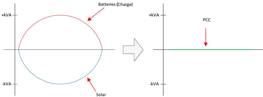
**Figure 2: Best Case - Battery Charging Matches Solar Output**
