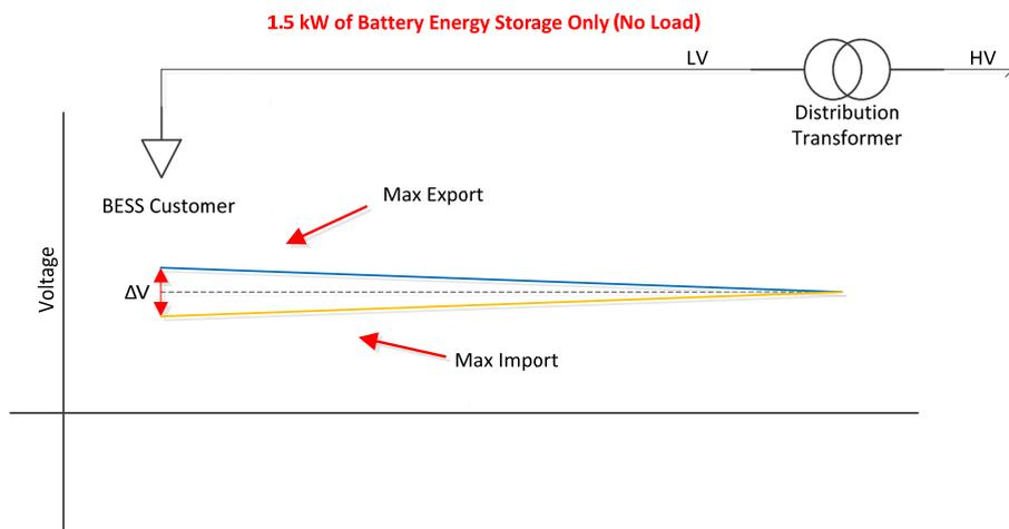
Figure 5: Premise with 1.5 kW of Battery Storage Only (No Load) - Change in Voltage Profile
