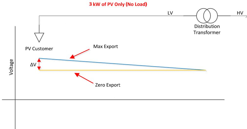
Figure 4: Premise with 3kW of PV (No Load) - Change in Voltage Profile
