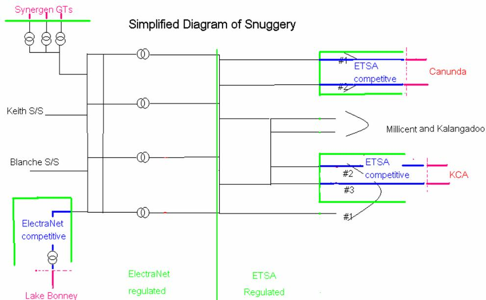
This simplified diagram shows the major connections at Snuggery substation. Connected at the substation are large generators (Lake Bonney and Synergen) and large embedded generator (Canunda), a large consumer (KCA) and a number of small consumers. Canunda exports more power than KCA and the other consumers guarantee to take at any time, indicating that Canunda needs access to the transmission system.
