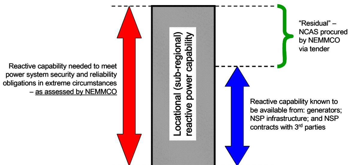
With respect to NCAS in the form of reactive power capability, the volume procured by NEMMCO on a locational (sub-regional) basis is currently determined as the residual between (see Figure E.8):
