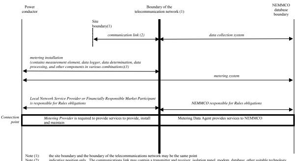
Note (2): indicative position only. The communications link may contain a transmitter and receiver, isolation panel, modem, database, other suitable technology, data processing and/or data transfer process(s). There may be more than one communication link within a metering installation.
