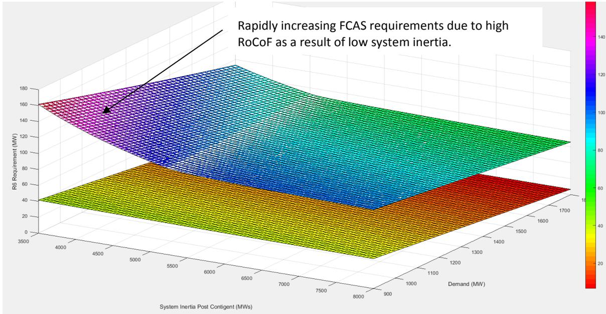
Figure 2 - Relationship between RoCoF, FCAS and Inertia
