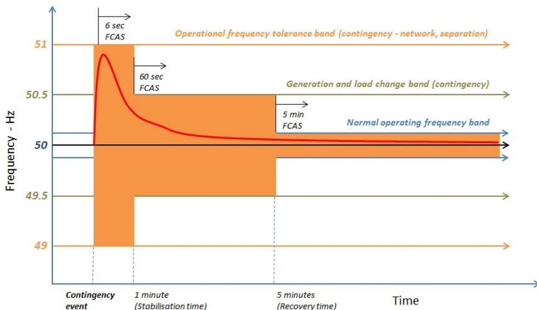
At any point in time, the steepness of the frequency curve represents the rate of change of frequency (RoCoF). As can be seen, the RoCoF is highest immediately following the occurrence of the contingency event.
