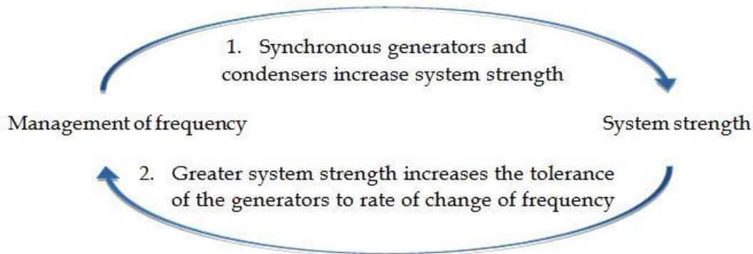
1. System strength is higher in the vicinity of the synchronous generators or synchronous condensers that provide inertia. As such, the provision of inertia may need to be distributed across the power system in order to prevent system strength being too high or too low in any particular location.
