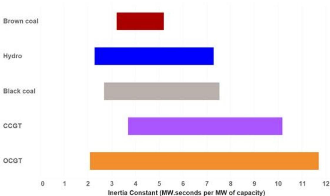
The relationship between inertia and capacity is not uniform. Some generating units provide significantly more inertia per MW of capacity than other generating units.
