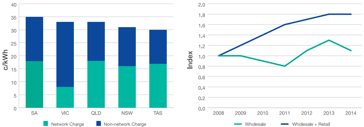
Figure 10: 2015 electricity price breakdown (left) and indexed wholesale and retail price (right) Source: CME.
