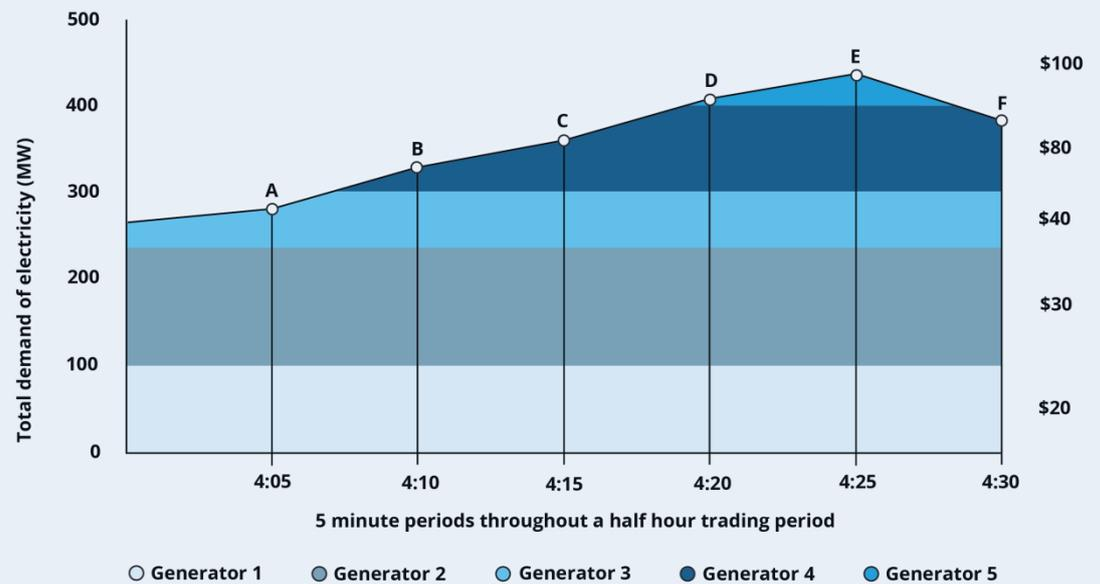
Bids to produce electricity received by AEMO are stacked in price order for each dispatch period. Generators are then progressively scheduled into production to meet demand, starting with the lowest cost generator.
