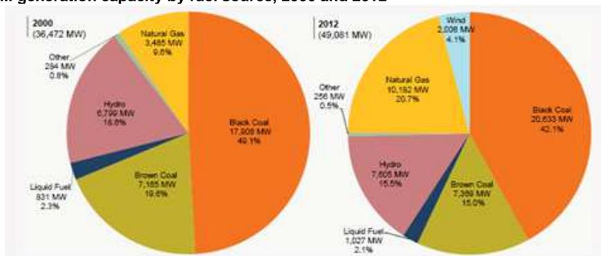
As shown above, wind generation increased dramatically between 2000 and 2012. Installed wind capacity in the NEM is over 2000 megawatts and climbing. While required build to meet the Renewable Energy Target, as shown below, equates to wind capacity of around 9155 megawatts by 2020, with around 8000 megawatts of hydro and 2700 megawatts of biogas.
