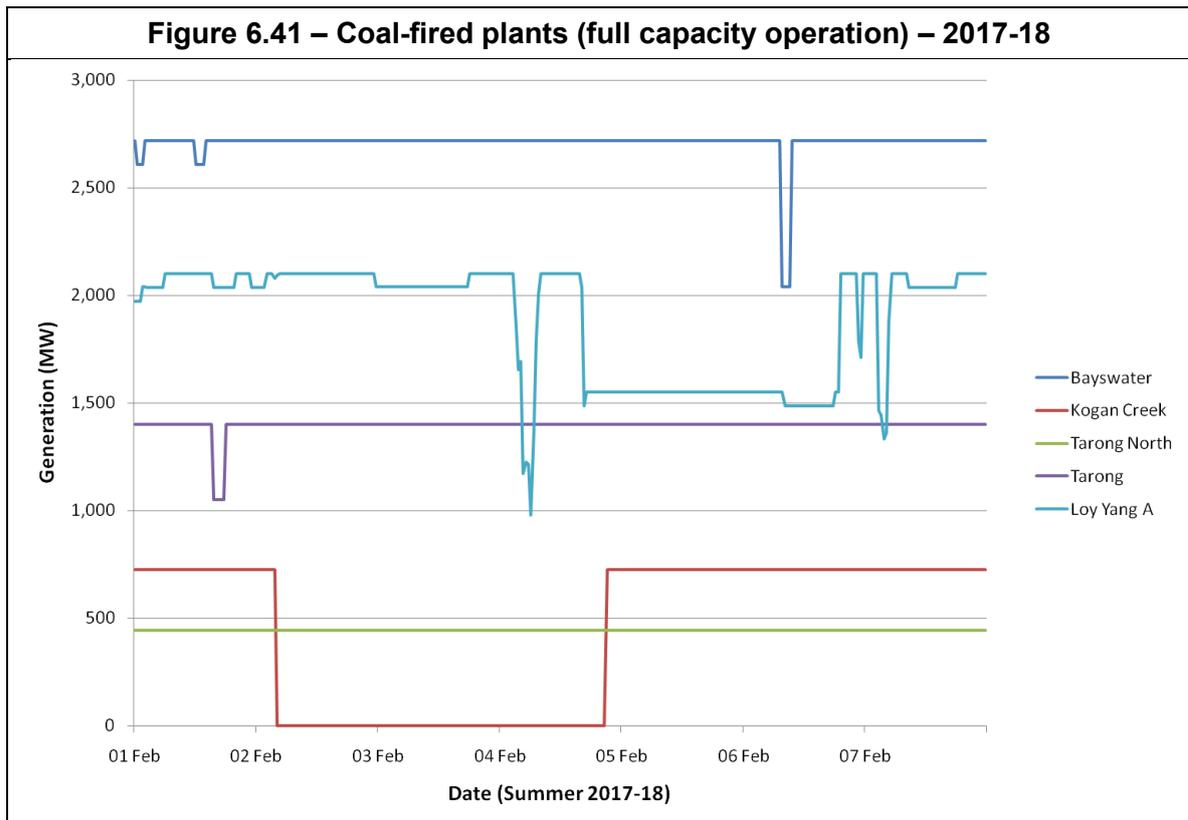
Kogan Creek experiences a forced outage during this period. Of the plants illustrated in Figure 6.41, Loy Yang A is the most impacted in operation by the CPRS and RET, due to its higher emissions factor (being a brown coal plant), and the high quantity of wind installed in Victoria over the course of the study (especially in the high banking case). Nevertheless, since it is one of the lowest emissions baseload plants in Victoria, it maintains high volumes (especially over the summer period).
