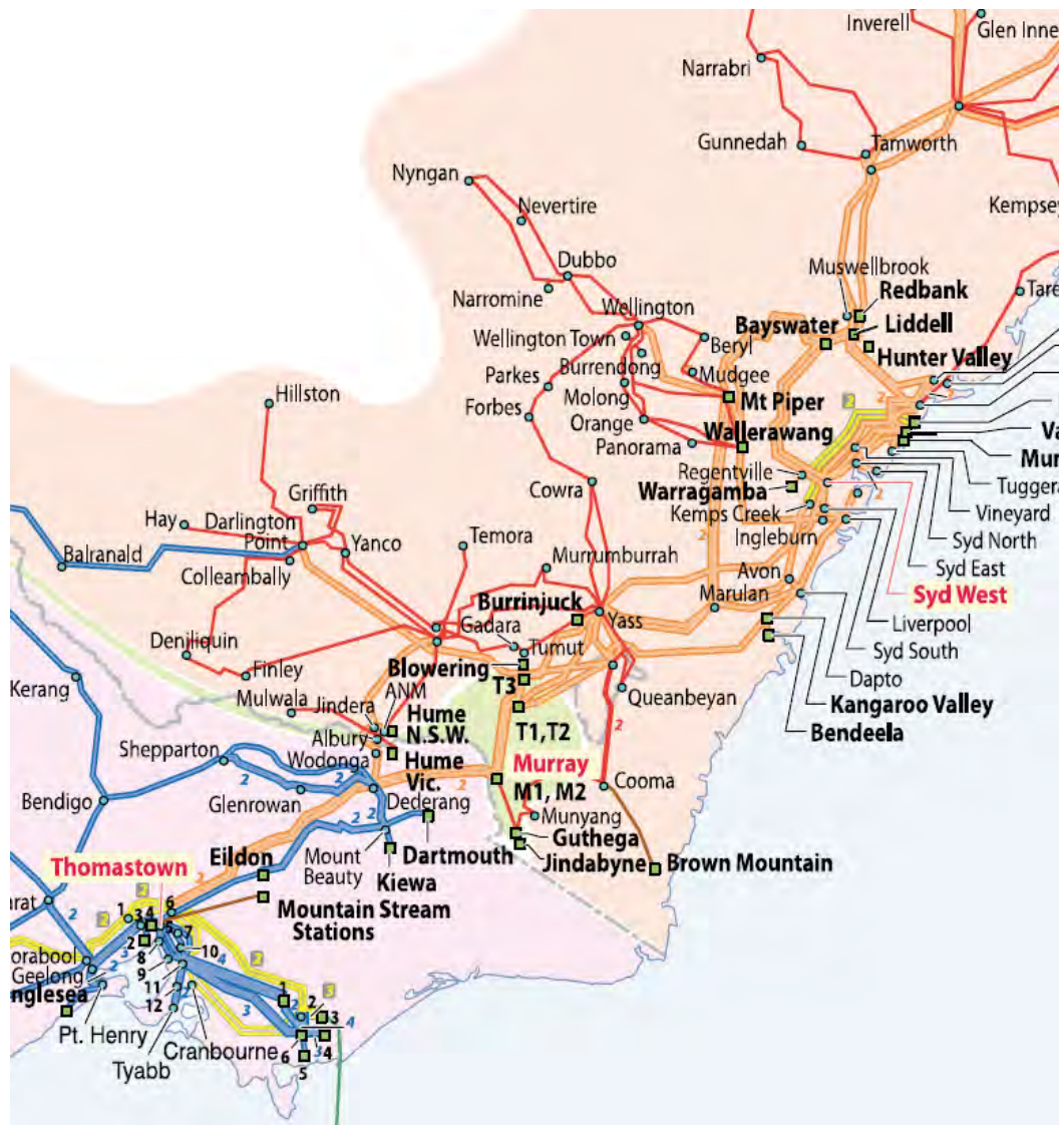
Figure F.1 Transmission network elements – Victoria-Snowy and Snowy-NSW Interconnectors
