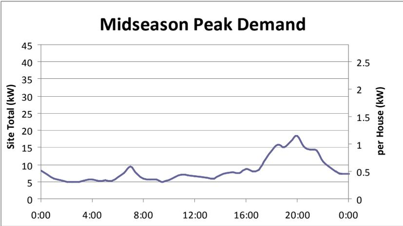
This data demonstrates the effect of taking the temperature sensitive loads and delivering these using the waste heat from the generation system. In this process green emission credits are also generated as it is recognised as a much lower greenhouse intense solution that typical grid supply. This is without any credits for distribution network augmentation deferral.
