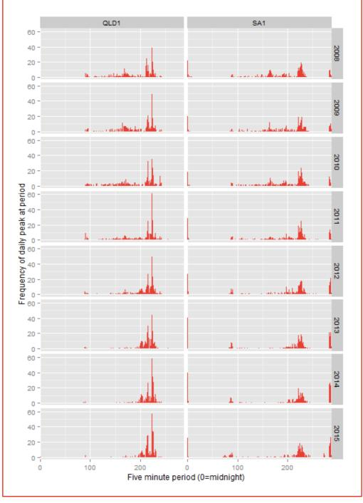
Figure 3: Peak shifting in Queensland and South Australia (net of solar PV)
