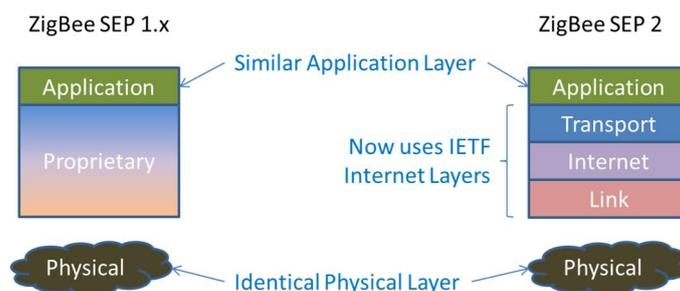
**Figure 14: Comparison of ZigBee SEP 1.x and SEP 2**
