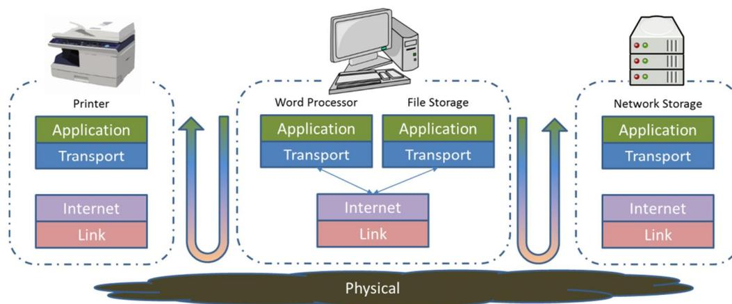
Figure 4: Example of Interoperability using the Internet Layers Model
