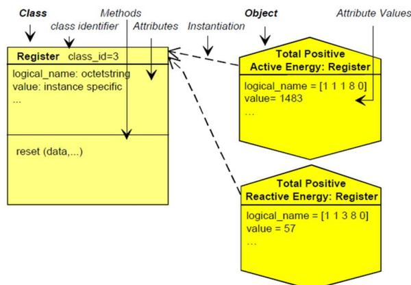
Figure 11: Example of two base objects available in COSEM Interface Classes
