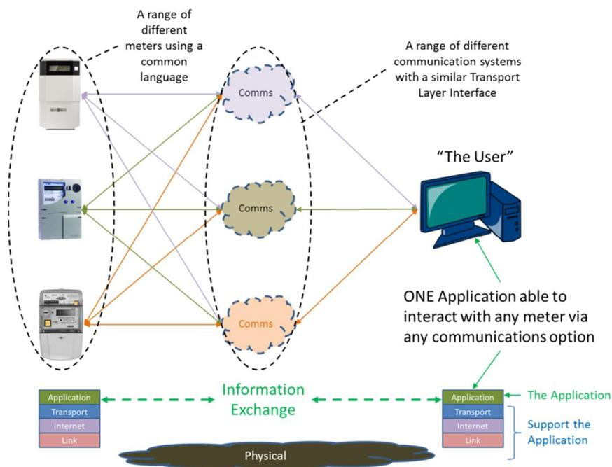
**Figure 5: Depicting how the Internet Layers Model supports meter interoperability**
