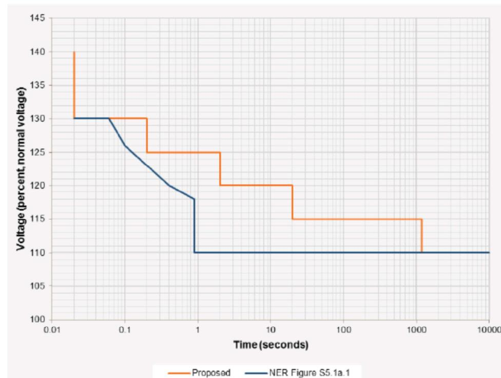
Figure 1: Proposed system standard for power frequency over voltage<sup>1</sup>
