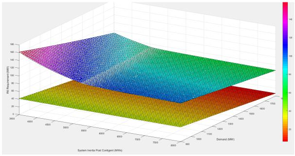
Figure 2 - Changes to FCAS requirements due to reduction contingency size
