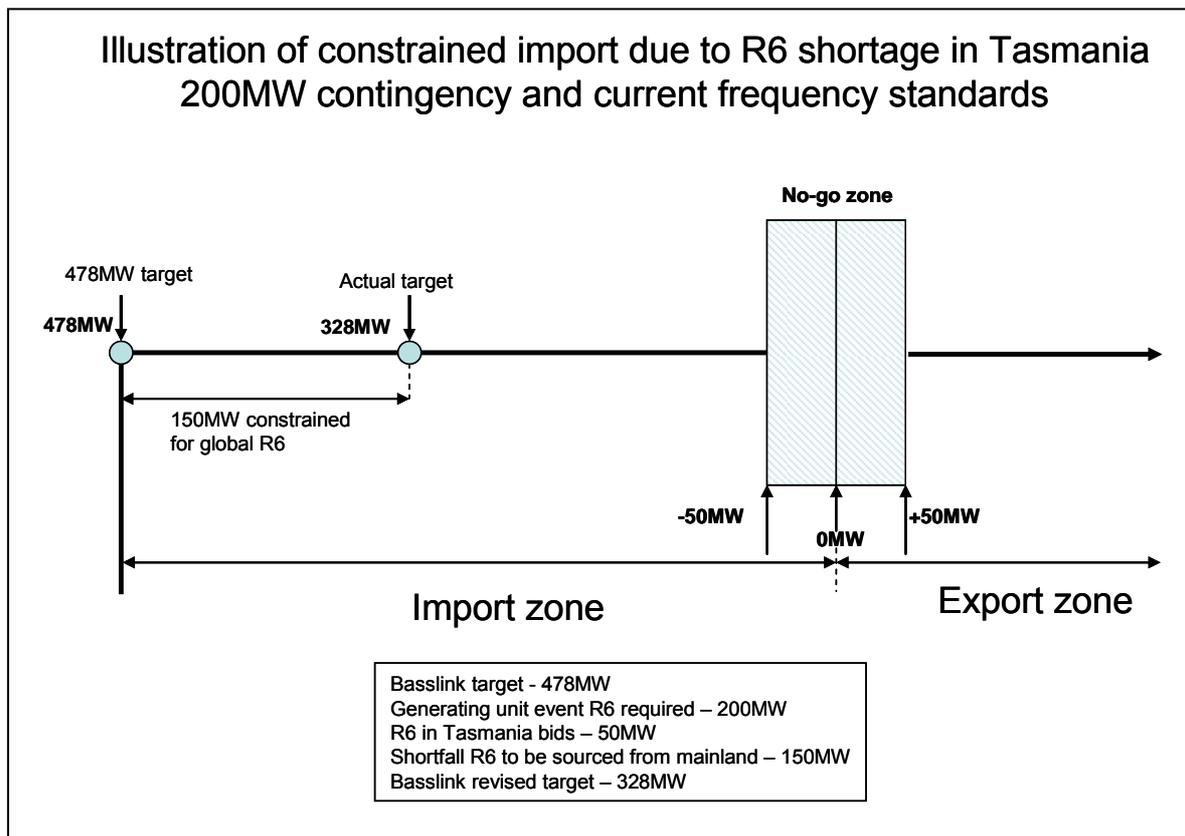
What should be noted in respect of Basslink is that, unlike an AC interconnector, Basslink has to traverse the no-go zone to reverse flow direction and also operate within hard availability limits (as set by MNSP owner). Basslink is typically required to reverse a number of times per day as prices vary across the NEM regions.
