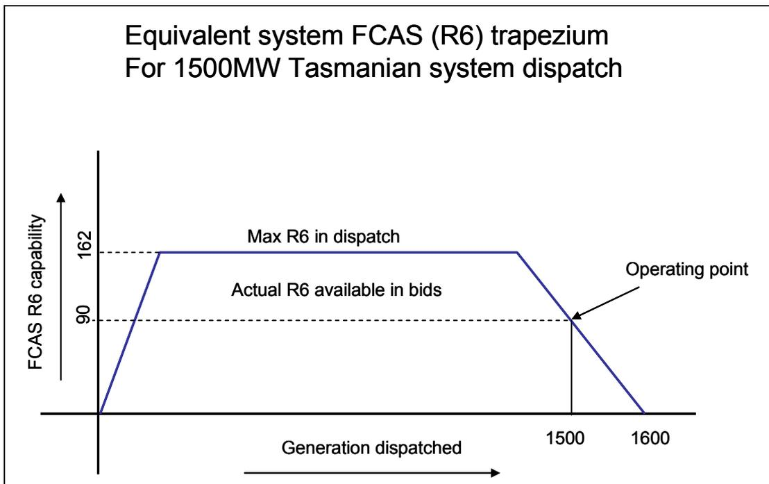
The three scenarios above illustrate what could be termed typical market dispatches of energy and FCAS to satisfy Tasmanian demands of 1000, 1250 and 1500 MW. The diagrams illustrate that under smaller Tasmania demands, the maximum R6 (trapezium aggregate) could be approximately 120 MW with only around 80 MW of R6 being available for the FCAS constraint equations due to the profile of the FCAS capability diagram (ie a tapering off at higher machine outputs).
