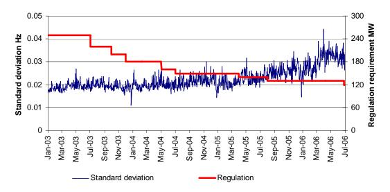
Figure 29 shows for each day, since 29 April 2005, the distribution of the measured frequency and the requirement for regulation FCAS (raise and lower) in Tasmania. A standard deviation below 0.05 Hz meets the Panel's standard.
