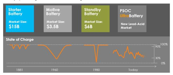
The fourth graph in the diagram represents a battery operating in continuous partial-state-of-charge. This is the operation required for variability management applications.
