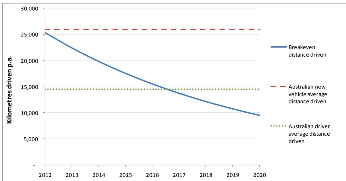
Note: Compares cost of running a petrol car to cost of running an electric car. For the purposes of this analysis, electric car running costs include electricity, battery, and the per vehicle share of capital and operating costs for an electric car charging network like Better Place
