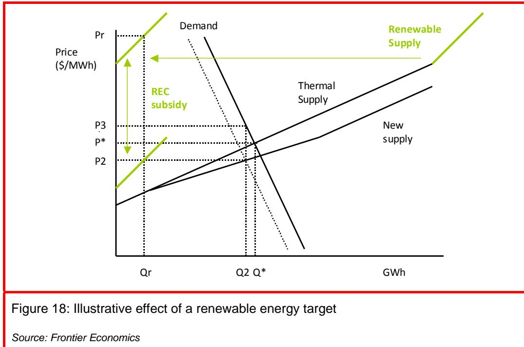
The introduction of the RET provides a targeted subsidy to renewable generators, allowing them to sell electricity at prices lower than their LRMC. This is because the sale of RECs provides revenue in addition to the wholesale energy price. This shifts the renewable supply to the bottom of the merit order, and shifts the thermal supply curve to the right. This is represented as New supply, which is a combination of thermal and subsidised renewable generation. Regarding Figure 18:
