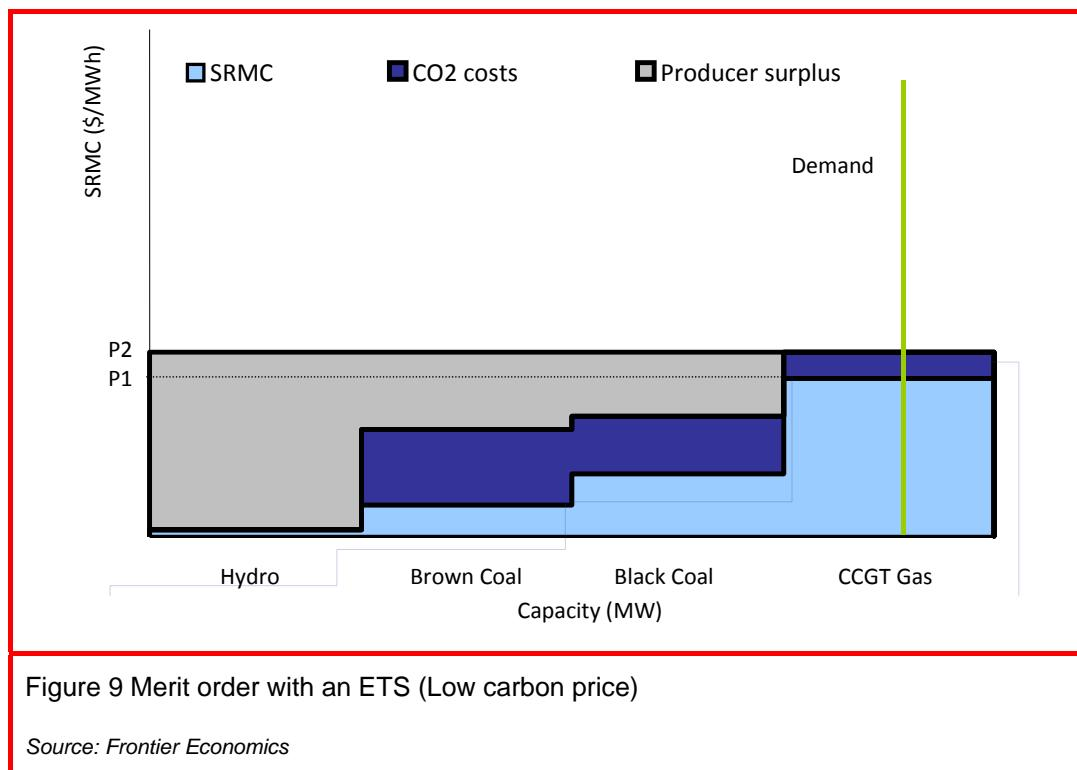
Although the change in price is the same for all generators, the change in cost is different for each generator according to their emissions intensity. Gas is able to pass-through its carbon cost. Black Coal and Brown Coal will experience a higher increase in costs, and their gross margins are reduced.
