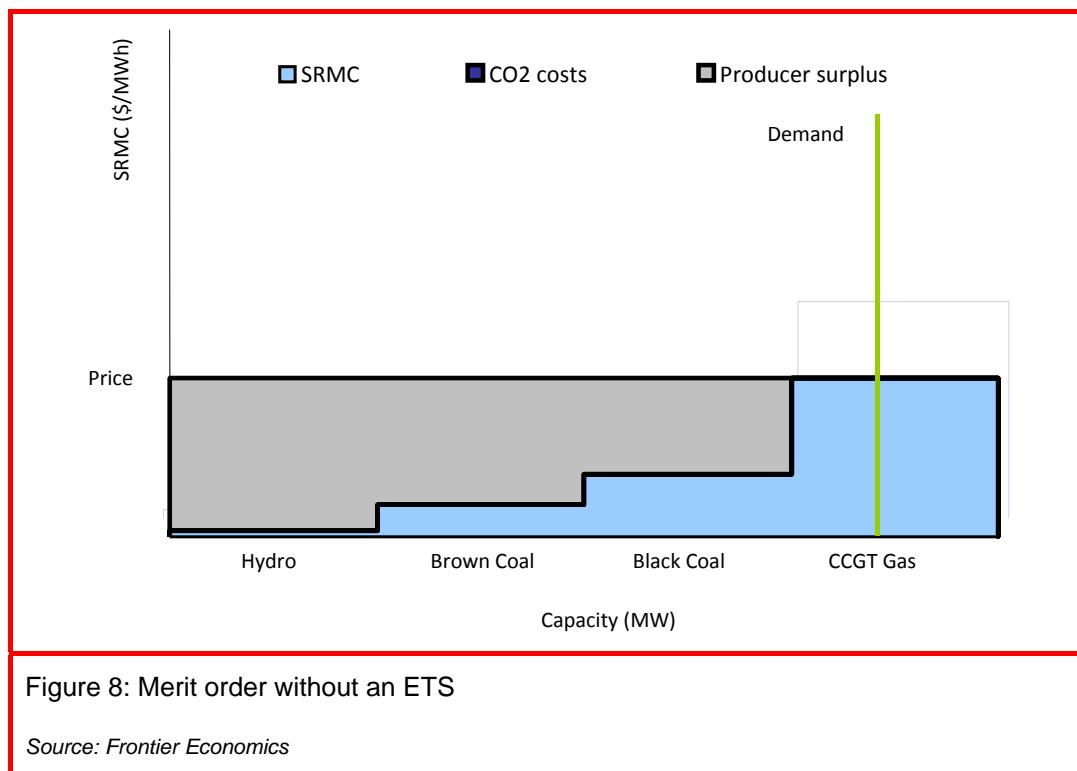
When an ETS is introduced, generators will add the carbon cost to their bids. However, the change in wholesale price depends on (a) the carbon price and (b) the emissions intensity of the marginal plant before and after the cost of carbon is introduced. Figure 9 presents the situation where the merit order is unchanged by the carbon price – gas remains the marginal generator and so the emissions intensity of the gas plant will determine the change in wholesale price ( $P_2 - P_1$ ).
