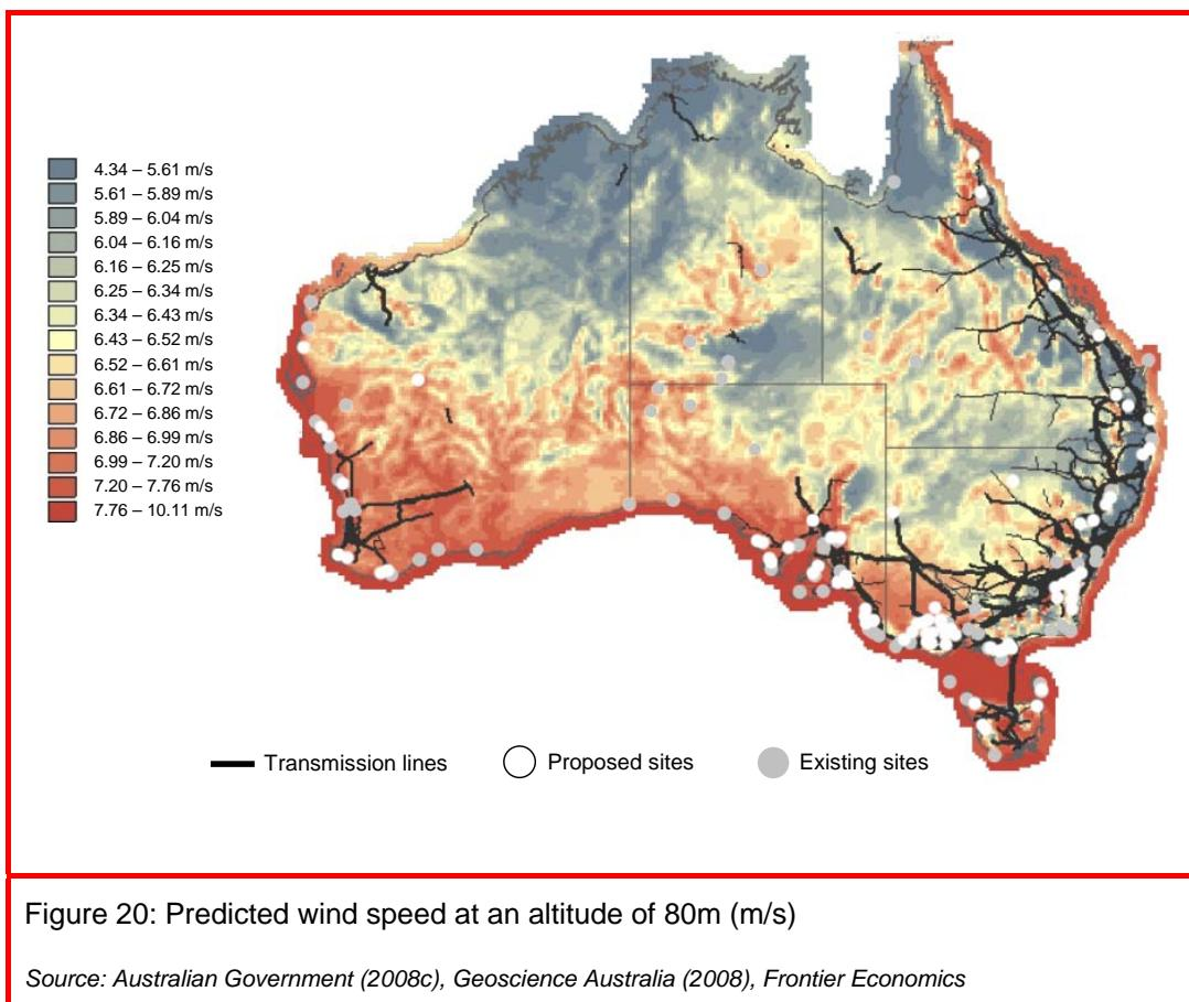
Figure 20: Predicted wind speed at an altitude of 80m (m/s)
