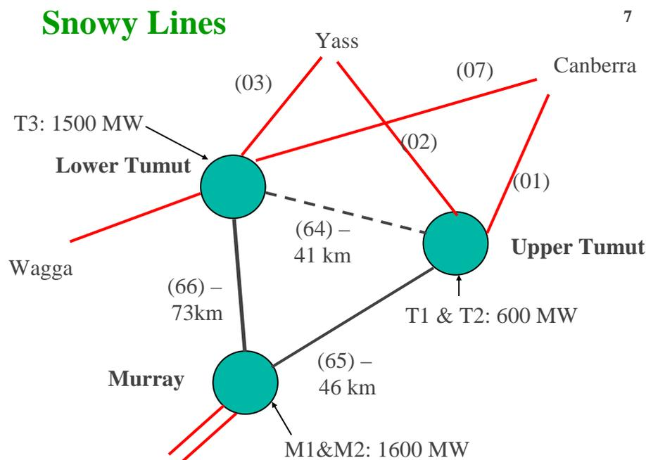
Note: Transmission line numbers are in brackets. The lines between Murray, Lower Tumut, and Upper Tumut are 330kV lines. M1 and M2 represent the Murray power stations and T1, T2, and T3 represent the Tumut power stations.
