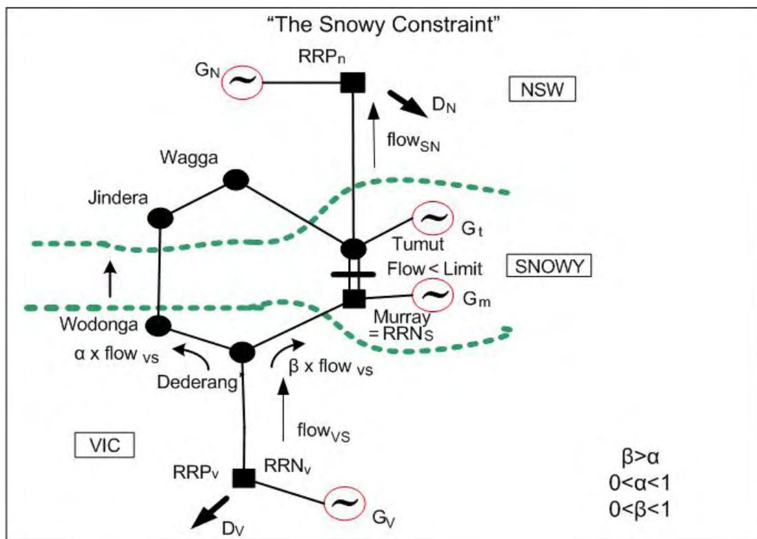
The limit on the Murray to Upper and Lower Tumut transmission lines ranges between 1,250MW and 1,350MW under normal network conditions. The congestion on these lines has increased since NEM start, especially since 2002, and the point of congestion is referred to as the Murray-Tumut constraint. This is a cutset constraint in the sense that it limits flows across a cutset of lines which also include the lines
