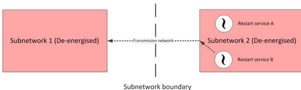
In this scenario, both subnetwork 1 and 2 are in a black system condition, and both restart services A and B are located in subnetwork 2. Restart service A has been contracted to provide restart services to subnetwork 2. Restart service B has been contracted to provide restart services to subnetwork 1.
