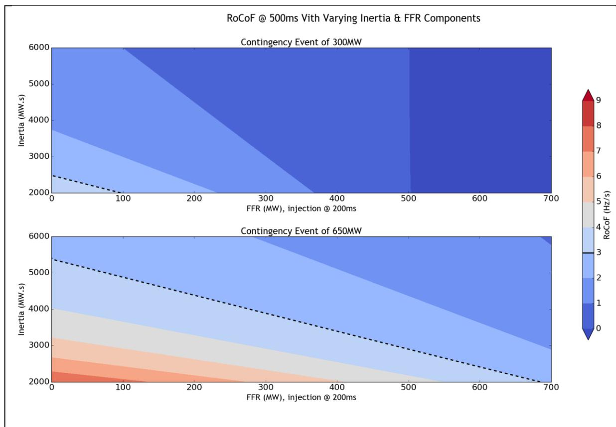
**Figure 2.** Comparison of different RoCoF levels at varying quantities of inertia and FFR for contingency sizes of 300MW and 650MW.
