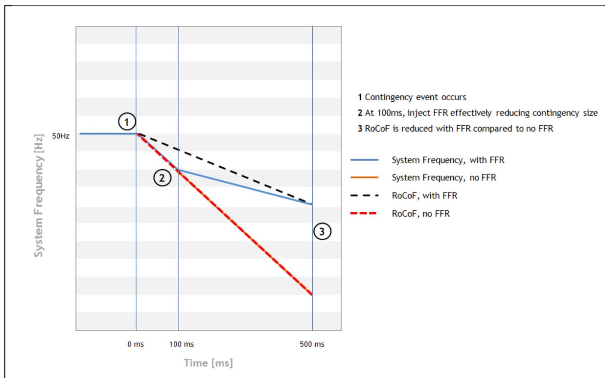
**Figure 1.** *Illustration of FFR contribution to managing initial rate of change of frequency to a contingent event.*
