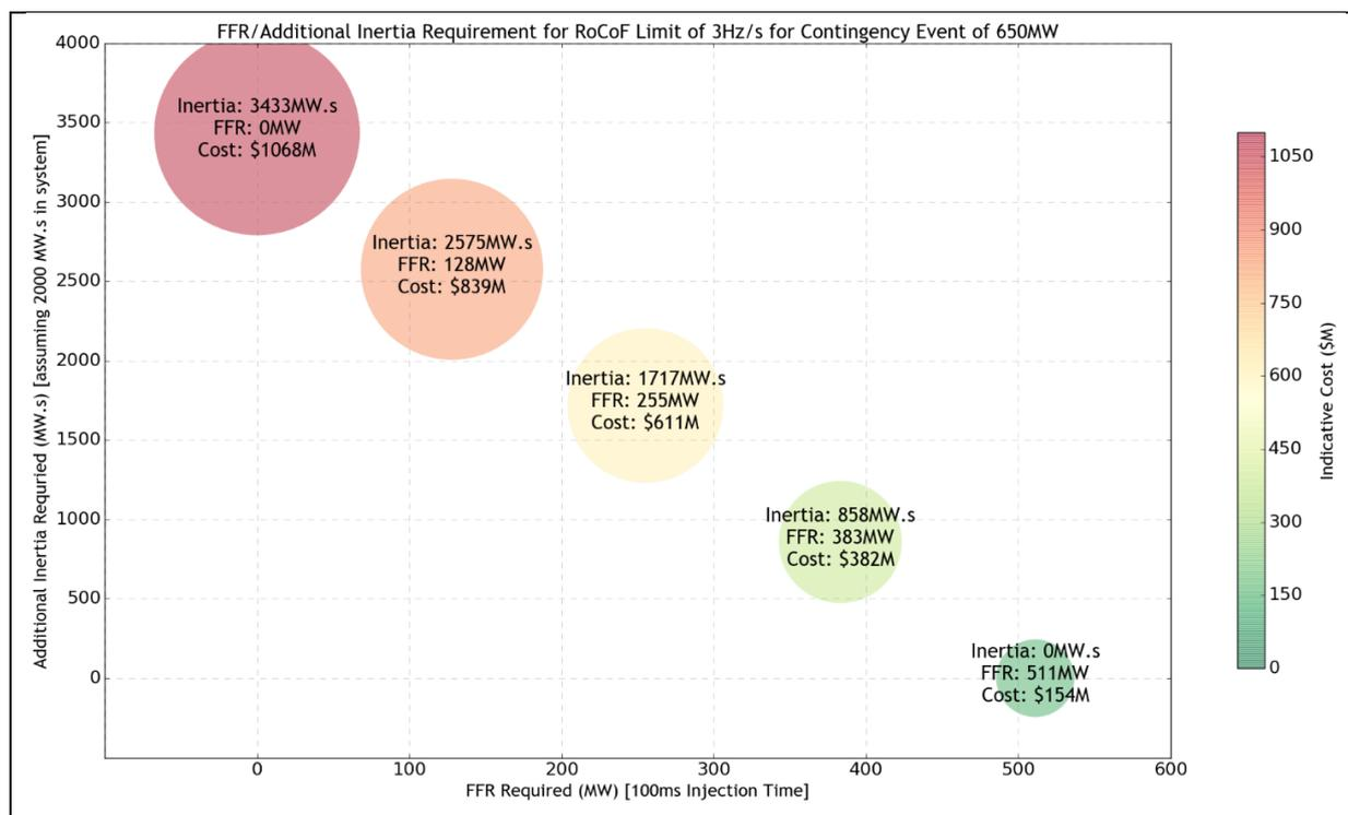
**Figure 4.** CAPEX comparison for varying blends of additional inertia and FFR to maintaining a 3 Hz/s RoCoF. (Note: Base inertia of 2000 MW.s)
