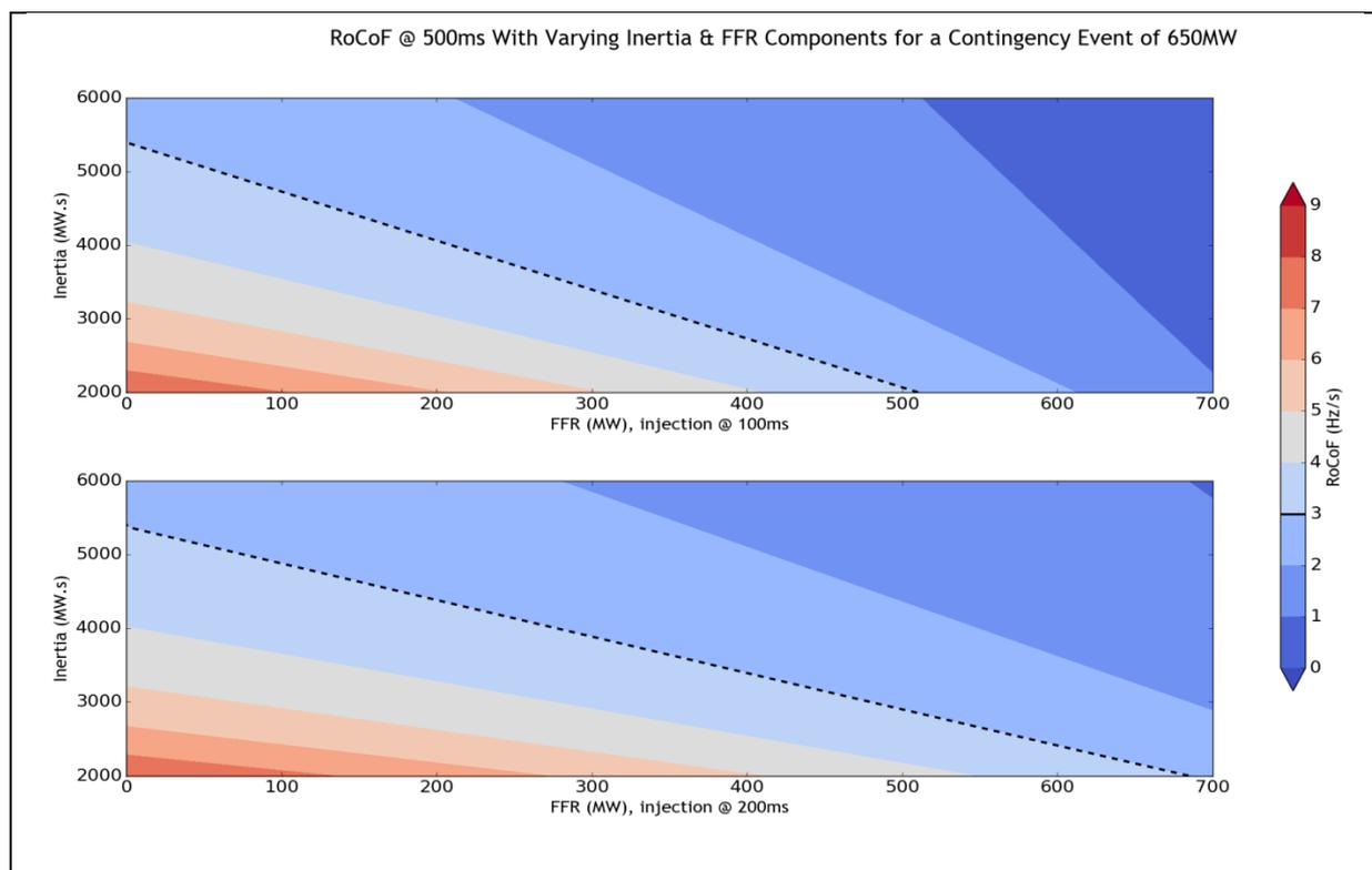
**Figure 3.** Comparison of relative impact of response times on RoCoF for a significant contingency event of 650MW.
