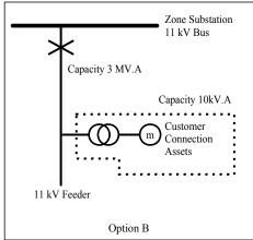
The 11 kV spur line has a large capacity compared to the expected *Distribution Customer maximum demand*. The *connection* charges associated with this asset would be abnormally high for a *Distribution Customer* of this size if this and the *distribution transformer* were included as *connection assets*.
