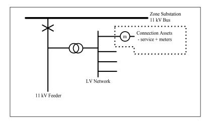
In this case there is virtually no choice, that is, the *connection assets* are the LV service lines plus *meters*, and all upstream *network* (LV mains, *distribution transformers* etc.). The *network coupling point* (boundary of *connection service* and *distribution service*) is the junction of the service mains and the LV mains. The *connection point* is the asset boundary between the service main and the customer's electrical installation.
