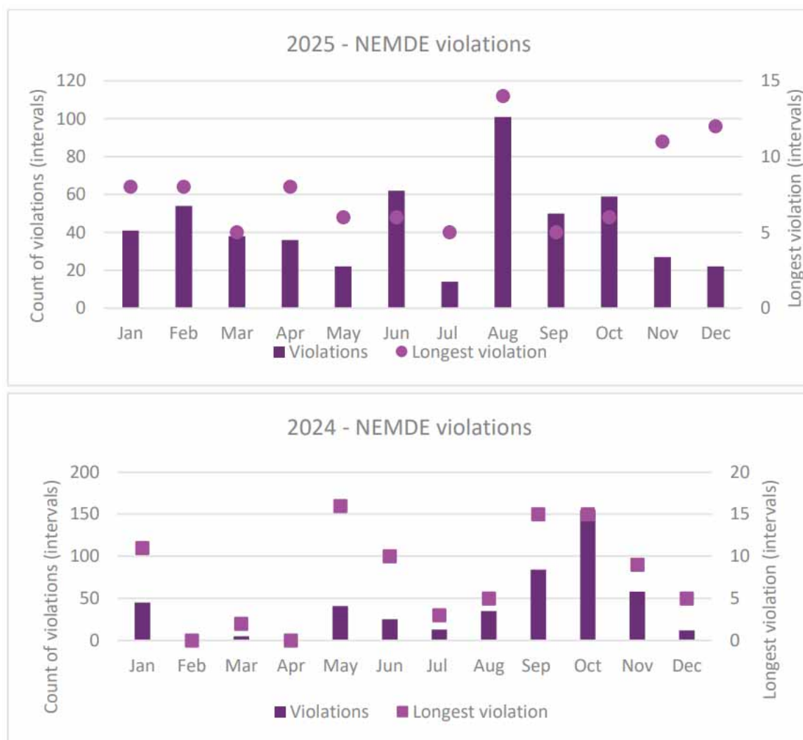
Figure 2.1: Number and length of inverter constraint violations in 2025 (top) and 2024 (bottom)
