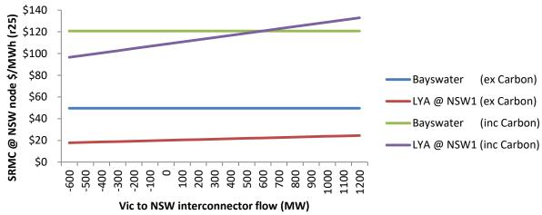
The chart shows that under current market conditions, with carbon unpriced, Loy Yang A can always out-compete Bayswater on price, even taking into account substantial marginal interconnector losses. From a carbon perspective, not only is Loy Yang A higher emissions, but those emissions are higher again when delivering power to NSW load under conditions of high northward interconnector flow.
