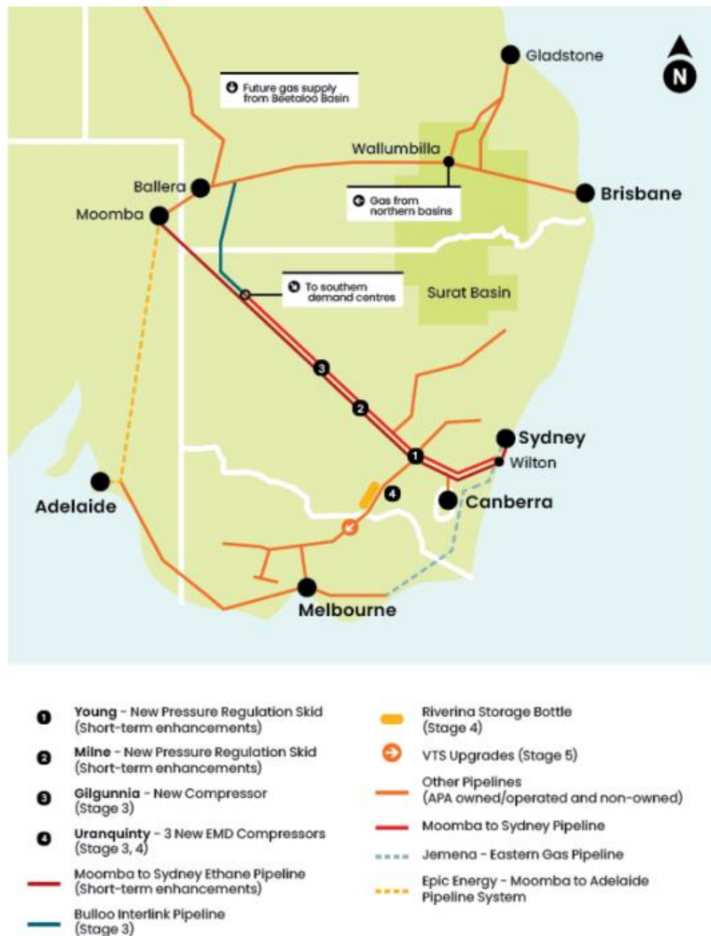
Figure 2: APA's East Coast Grid expansion plan
