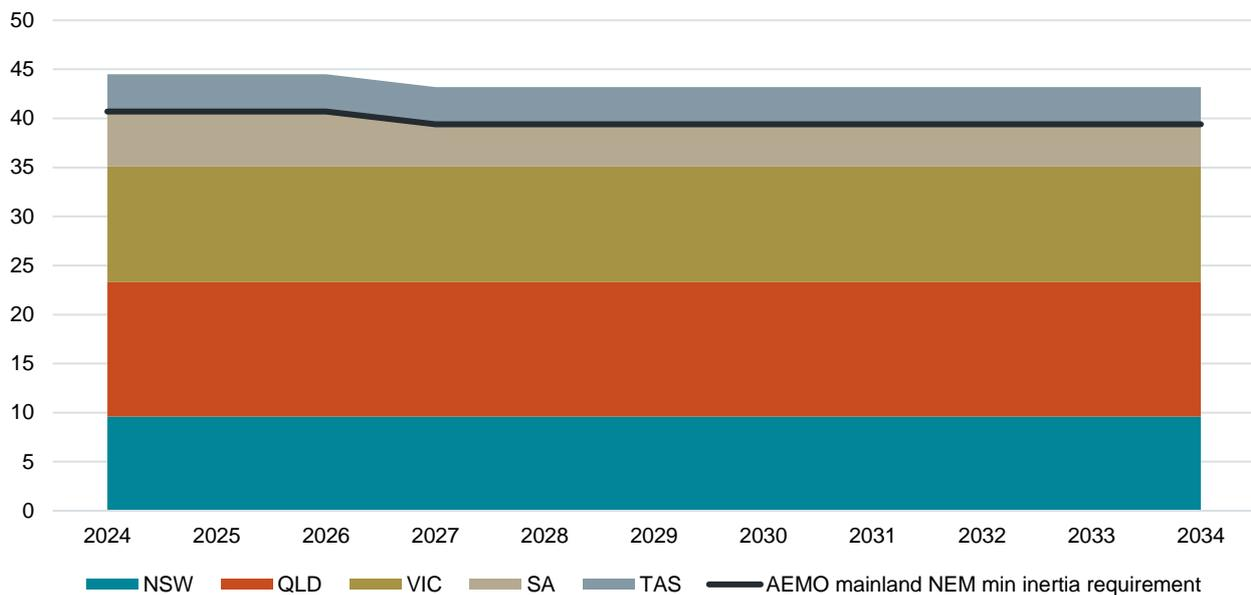
The black line represents the minimum inertia requirement for the mainland NEM projected by AEMO through to 2034. The black line sits at 39.4 GWs following the commissioning of Project Energy Connect (PEC), which the chart above assumes will occur in 2027. AEMO's minimum inertia requirement for the mainland NEM is 40.7 GWs before the commissioning of PEC.
