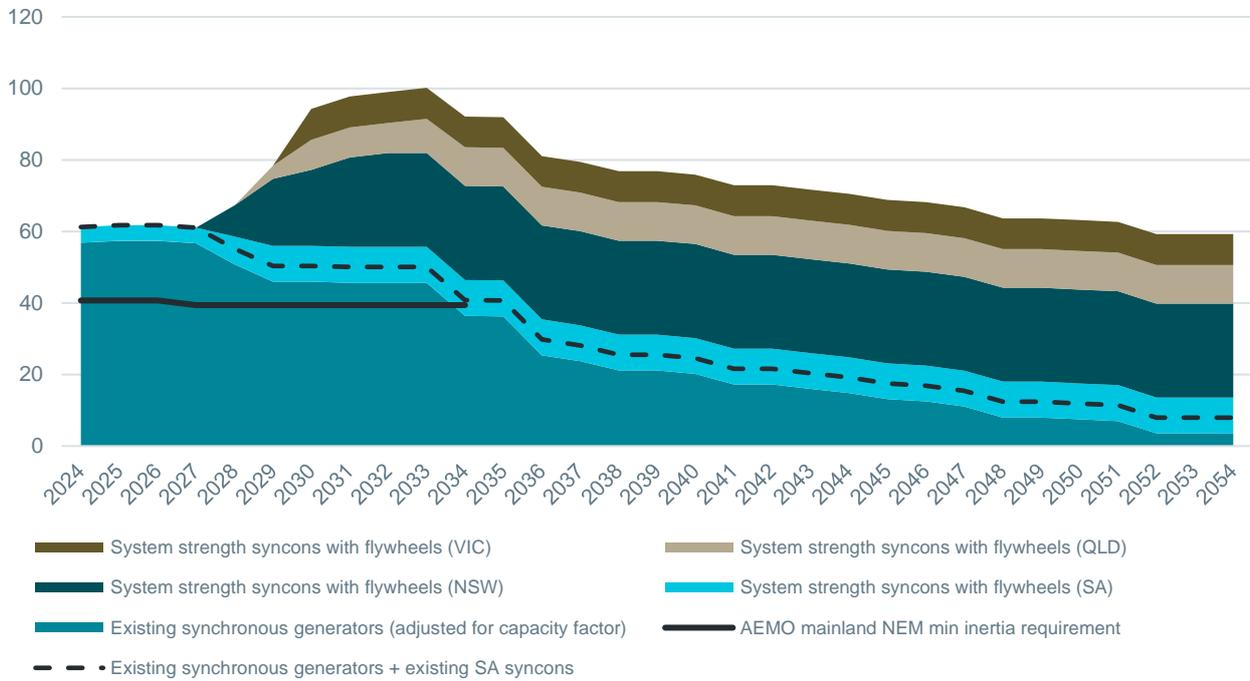
Figure 2.4: Existing generator average inertia plus system strength synchronous condensers with flywheels (low scenario)(GWs)
