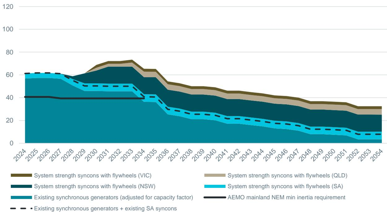
The analysis is consistent with a conclusion that system inertia capacity in the NEM is unlikely to fall below minimum requirements in the short to medium term, given anticipated investment in synchronous condensers (with flywheels) or alternative system strength technologies that may also be adapted to provide inertia.
