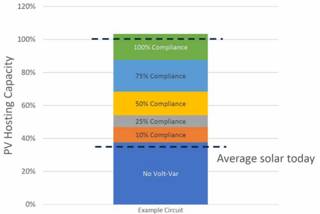
Figure 2.3: Incremental improvement in PV hosting capacity as compliance increases
