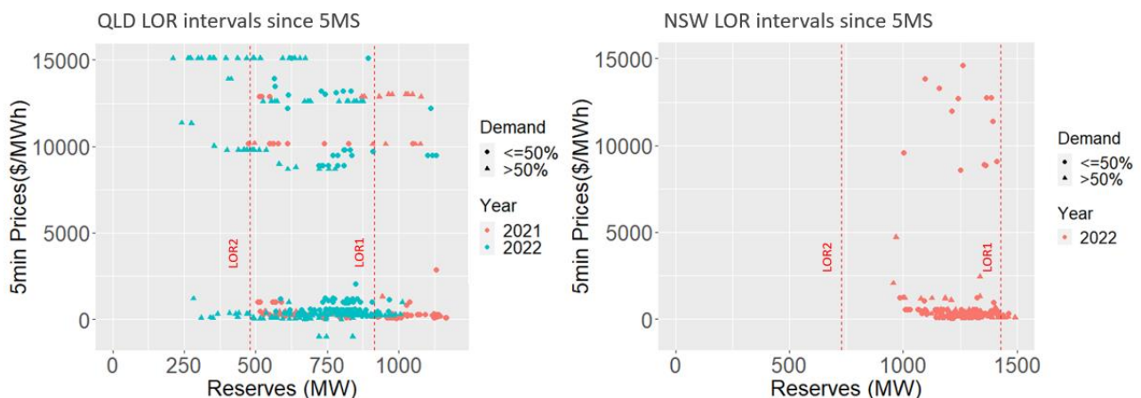
Figure 9 Price vs Reserve data for QLD (left) and NSW (right) LOR intervals following the implementation of 5-minute settlement. There is a significant number of intervals, even in the short period of time since 5MS, with low reserves (<LOR1), low demand (<50th percentile, [circles]), and suppressed prices (significantly below MPC).
