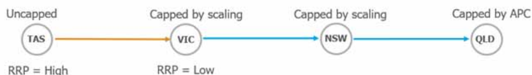
Figure 2.1: How Basslink incurred a loss in the spot market during the June event when the administered price cap applied in Queensland.
