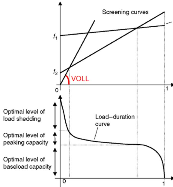
Figure 5. Illustration of classical screening curve analysis (adapted from Biggar and Hesamzadeh<sup>22</sup>).
