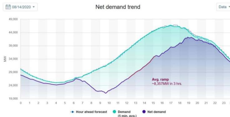
Figure 3. Hour-ahead forecast and real-time demand and net demand in California, 14 August 2020 (Source: Joskow’s presentation at MIT, 5 October 2020, taken from California Independent System Operator<sup>19</sup>)
