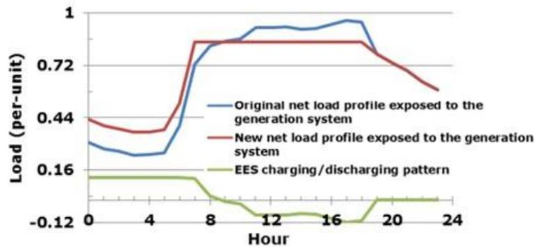
Figure 7. Illustration of the impact of storage on the change in the net load profile, based on a peak reduction storage control strategy (Source: adapted from Y. Zhou<sup>25</sup>).
