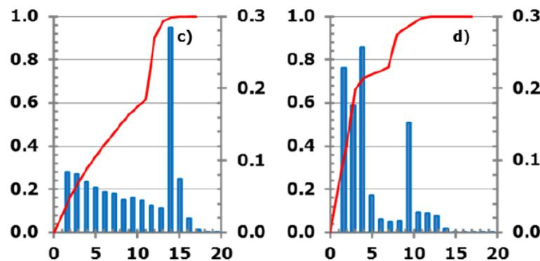
Figure 8. Probability distributions of the duration (in hours) of individual capacity shortfall events with storage (left) and without storage (right). The red curves represent the cumulative probability distribution functions (vertical axis on the left-hand side), and the blue histograms are the probability density functions (vertical axis on the right-hand side). (Source: adapted from Y. Zhou<sup>25</sup>).
