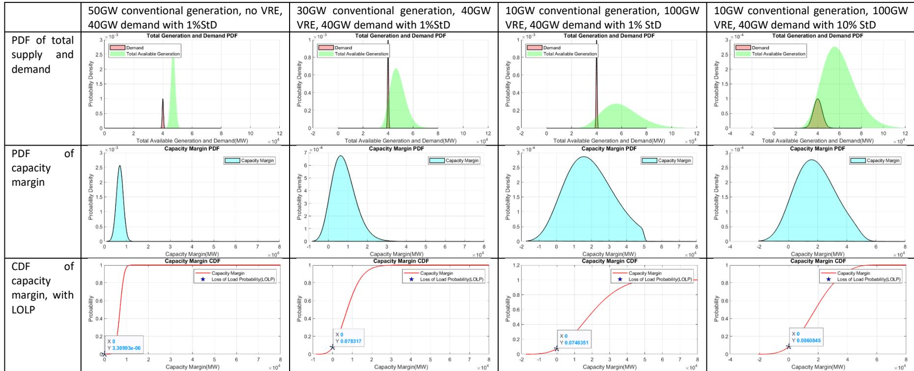
Figure 2. Qualitative illustration of changes in shape of probability density function (PDF) and cumulative distribution function (CDF) of supply, demand, and capacity margin, overall describing a changing risk profile, while the system becomes more decarbonized.
