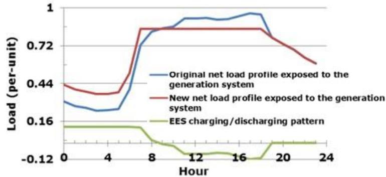
Figure 7. Illustration of the impact of storage on the change in the net load profile, based on a peak reduction storage control strategy (Source: adapted from Y. Zhou<sup>25</sup>).
