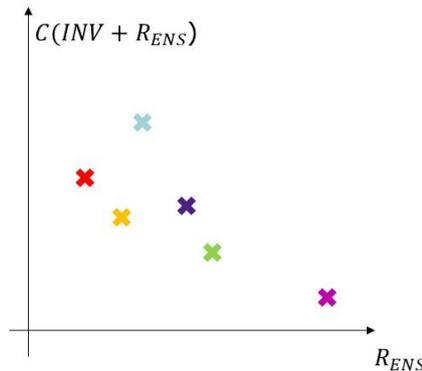
Figure 20. Illustration of efficient reliability level plots for a composite reliability metric  $R_{ENS} = w \cdot EENS + (1 - w) \cdot \alpha\%CVaR_{ENS}$ , for a given level of the weight  $0 \leq w \leq 1$ .
