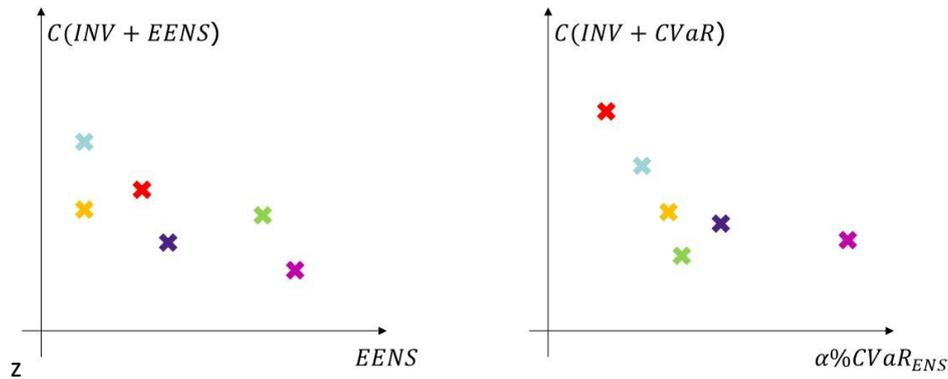
Figure 19. Illustration of efficient reliability level plots for (left) expected energy not supplied ( $w=1$ ) and (right)  $\alpha\%$  conditional value at risk of the energy not supplied ( $w=0$ ).
