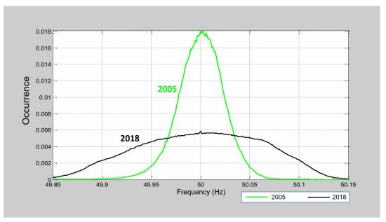
Historically in the NEM, only synchronous generators, such as coal, gas and hydro, have provided primary frequency response. However, non-synchronous generators such as wind, batteries and solar PV, can also provide primary frequency response.
