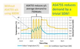
The same testing shows in identical conditions, but without AS4755, the air-conditioner would only have been using 800Watts. The CSIRO testing therefore reveals the actual demand reduction is only 50Watts, or 6% of the claimed demand reduction.
