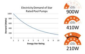
The inclusion of pool pumps in the Government's energy labelling scheme encourages consumers to install energy efficient variable speed pumps. In addition to significant energy savings (often exceeding \$400 a year [Ref 6]). The above figure shows the more stars the lower the electrical demand. Highly rated pool pumps now uses less than 200Watts. Continuing to claiming a demand reduction of 1000W for each pool pump is no longer valid.
