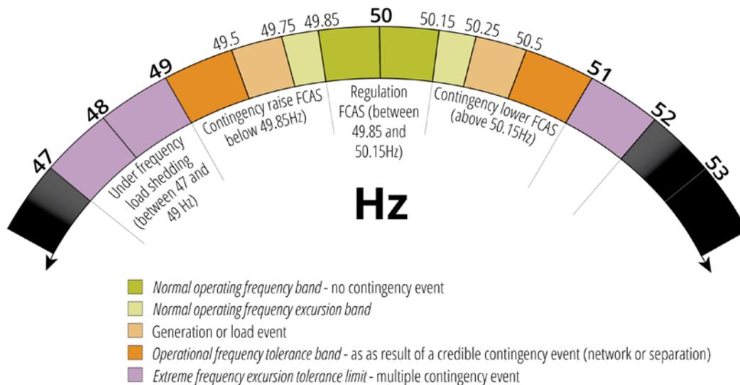
Figure 1. Frequency Bands for the mainland NEM and the zones of operation for ancillary services and under-frequency load shedding schemes
