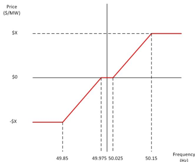
Figure 5. Example deviation price function for frequency control
