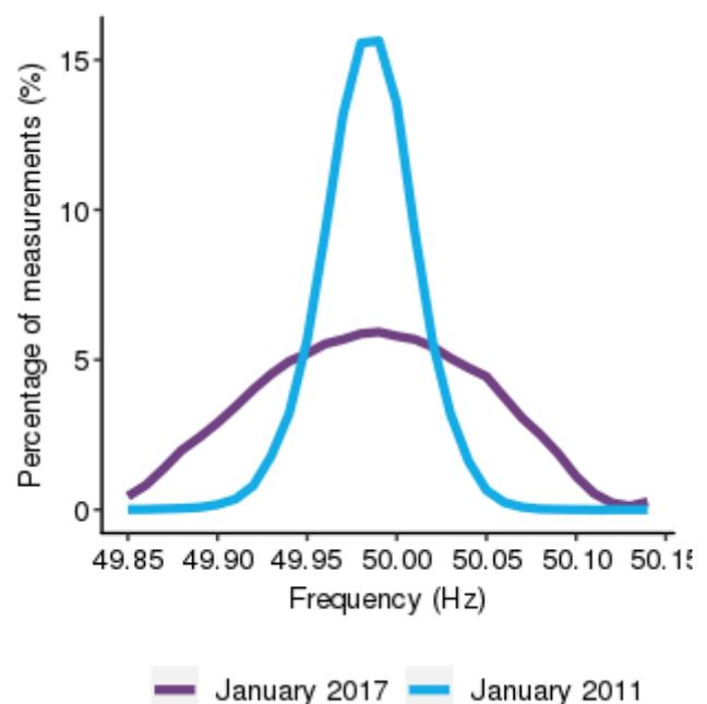
Figure 2. Frequency distributions based on measurement at four second intervals by AEMO for January 2011 and January 2017
