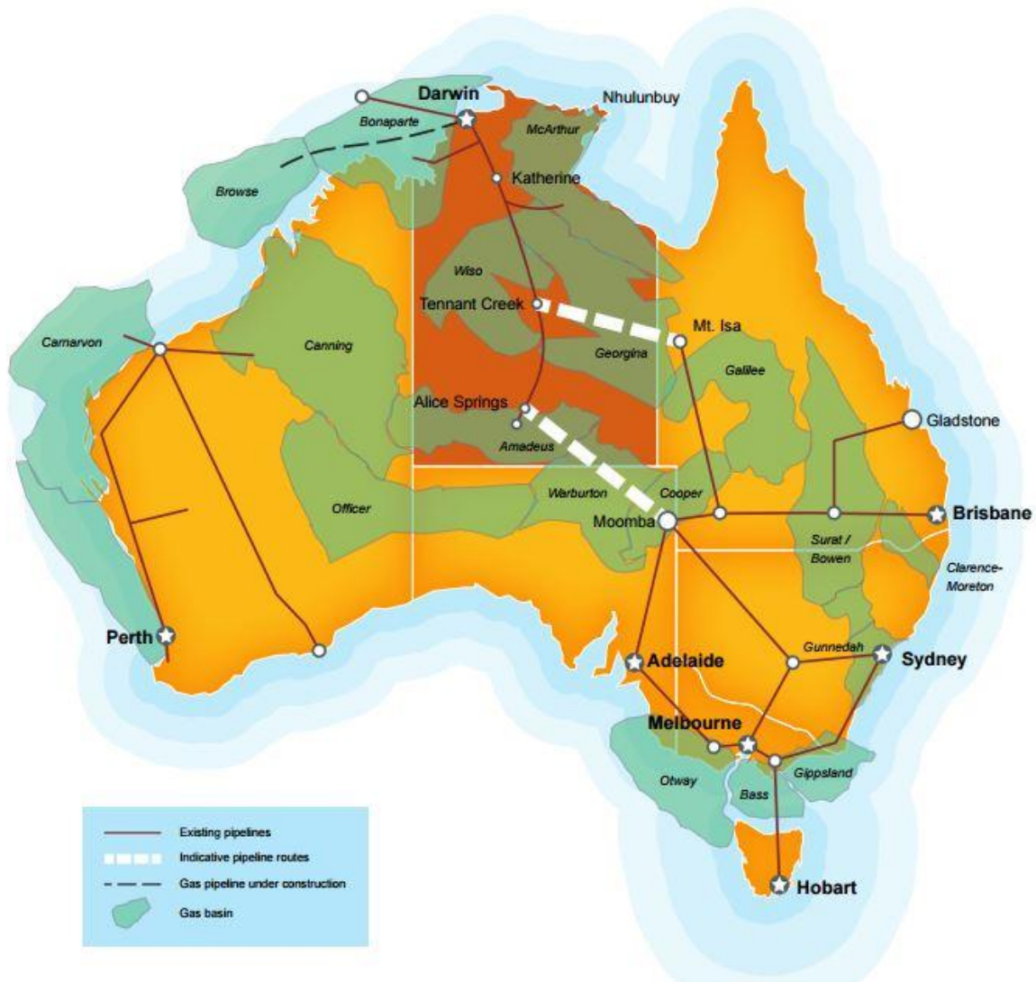
Figure 2.1: Proposed route of the NEGI connecting the north and east gas markets
