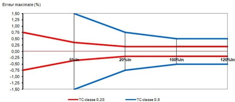
Figure 1: Current transformer accuracy
