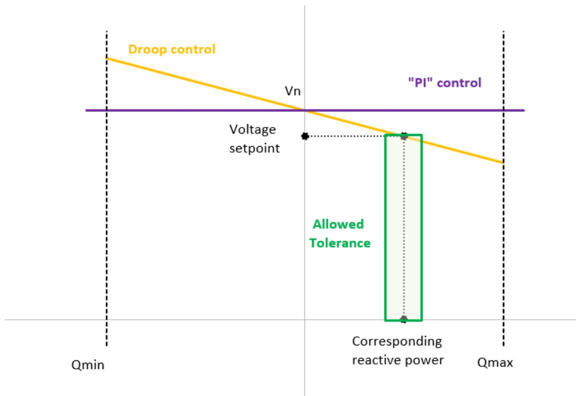
Figure 4: Example of voltage droop control
