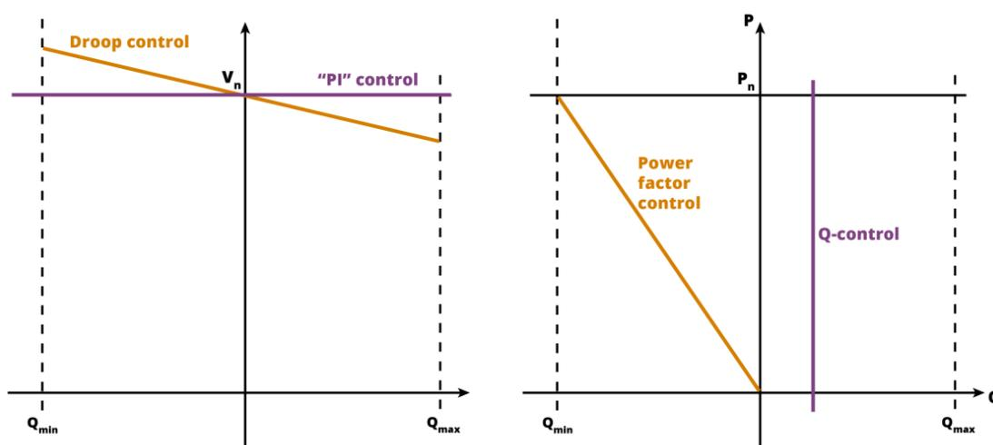
Figure 3: Reactive power control modes – voltage, reactive and power factor control [Draft Rule Determination, page 119]
