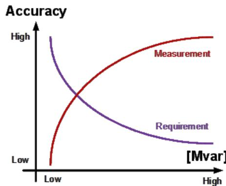
Figure 2: The relationship between the required accuracy of the reactive power and the accuracy of the measurement device
