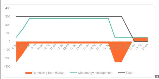
The solar panels cut power costs during the day where power use is the highest. Later in the afternoon on this sample day spot energy prices increase to high levels. Flow Power's kWatch® Intelligent Controller switched off the air/reduce conditioning thereby pushing unused solar generation into the grid. This resulted in this school receiving the high market price for its exported energy and also supporting the power grid.
