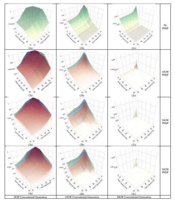
Figure 6. LOLP as a function of available conventional generation and PHSP storage. The three surfaces represent energy storage duration associated with power capacity: 6h (green),12h (blue) and 24h (red) (Source: Liu and Mancarella<sup>24</sup>).
