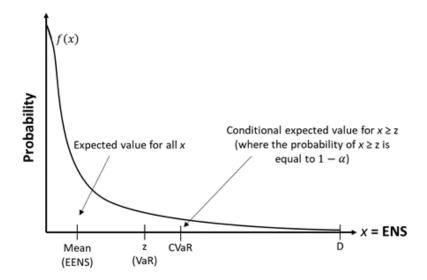
Figure 13. Probability distribution of energy not supplied, highlighting the "mean" metric (EENS) and "tail" metric (CVaR), adapted from Moreno *et al*<sup>30</sup>. 1- $\alpha$  indicates the size of the considered set of worst cases, *VaR* (or *z*) is Value at Risk, *CVaR* is Conditional Value at Risk, *D* is maximum demand, *x* is Energy Not Supplied (ENS), and the Mean value is the Expected Energy Not Supplied (EENS).
