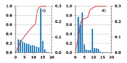
Figure 8. Probability distributions of the duration (in hours) of individual capacity shortfall events with storage (left) and without storage (right). The red curves represent the cumulative probability distribution functions (vertical axis on the left-hand side), and the blue histograms are the probability density functions (vertical axis on the right-hand side). (Source: adapted from Y. Zhou<sup>25</sup>).
