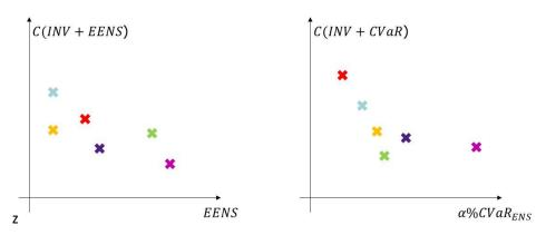
Figure 19. Illustration of efficient reliability level plots for (left) expected energy not supplied (w=1) and (right)  $\alpha$ % conditional value at risk of the energy not supplied (w=0).
