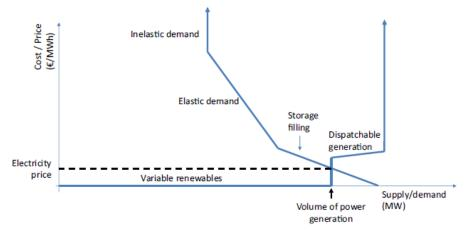
Figure 14. Effect of storage and demand side flexibility on electricity prices with high VRE output (Source: De Vries and Jimenez<sup>26</sup>).
