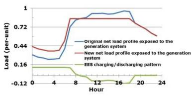
Figure 7. Illustration of the impact of storage on the change in the net load profile, based on a peak reduction storage control strategy (Source: adapted from Y. Zhou<sup>25</sup>).
