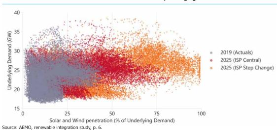
Figure 4.3: Instantaneous penetration of wind and solar generation, actual in 2019 and forecast for 2025 under ISP Central and Step Change generation builds
