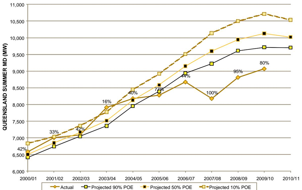
Figure B-10 shows the Queensland one-year-out and two-year-out energy back assessments. The yearly energy projections assume average weather conditions, while the actual data reflects weather conditions that actually occurred.
