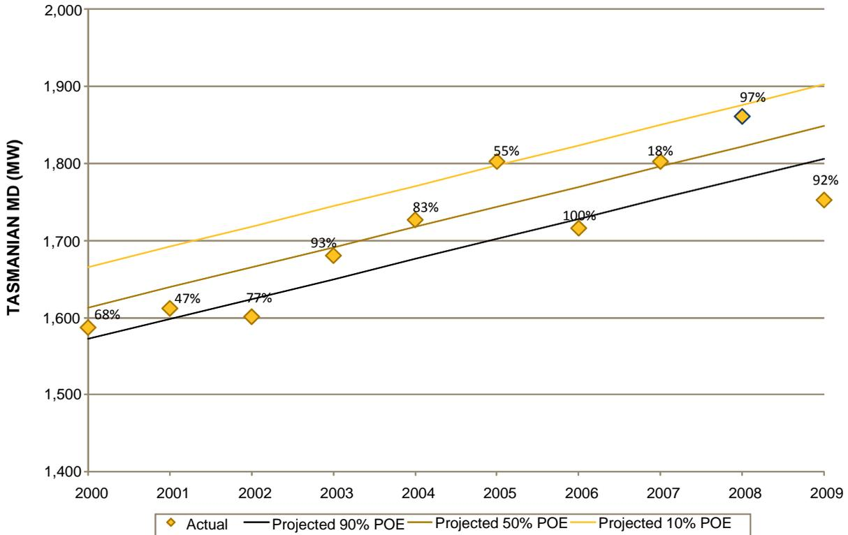
Figure B-33 shows actual MDs and estimated demand levels at standardised POEs. The actual MDs are mostly contained within the 90% POE and 10% POE estimated values. However, in relation to the assessed POE levels, the actual MDs are not generally well aligned. This reflects the following aspects of the data construction:
