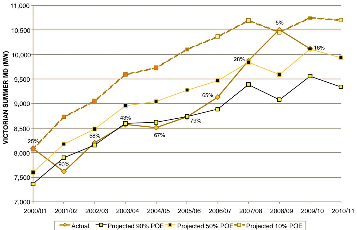
Figure B-21 shows the Victorian one-year-out and two-year-out energy back assessments. The yearly energy projections assume average weather conditions, while the actual data reflects weather conditions that actually occurred.
