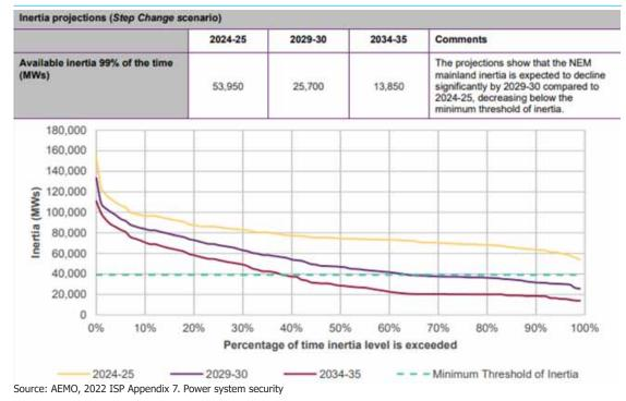
Figure 2.1: AEMO step change inertia projections
