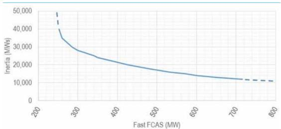
Figure 3.1: Stylised plot of inertia-FFR tradeoff
